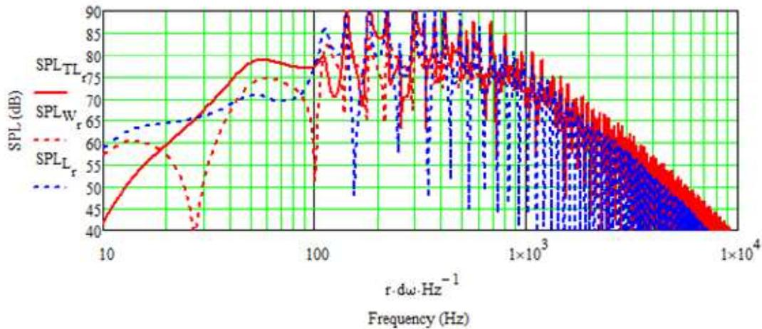
Figure 13 : Comparison of SPL Responses for 10 : 1, 1 : 1, and 1 : 10 Constant Volume Transmission Lines w/ 0.75 lb/ft<sup>3</sup> of Fiber Stuffing
