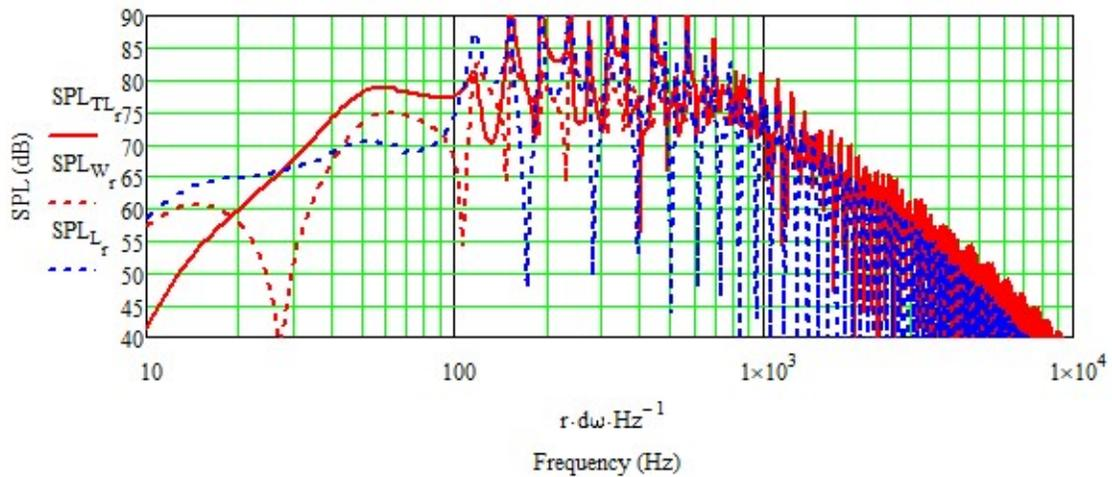
Digging a little deeper into the SPL plots presented in Figures 3, 4, and 5; the simulation results were replotted between 10 and 1000 Hz. The SPL, electrical impedance, driver cone displacement, and port or terminus oscillating air velocity are shown from top to bottom respectively in Figures 6, 7, and 8. Again these results do not include any fiber stuffing so enclosure resonances are easily identified in the curves.
