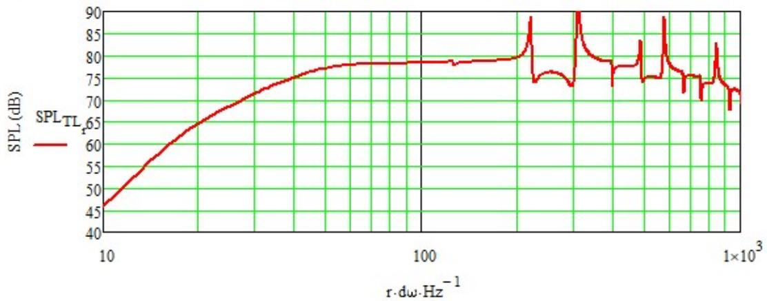
**SPL Response of a 10:1 Tapered Transmission Line Enclosure w/ Fiber Stuffing**
