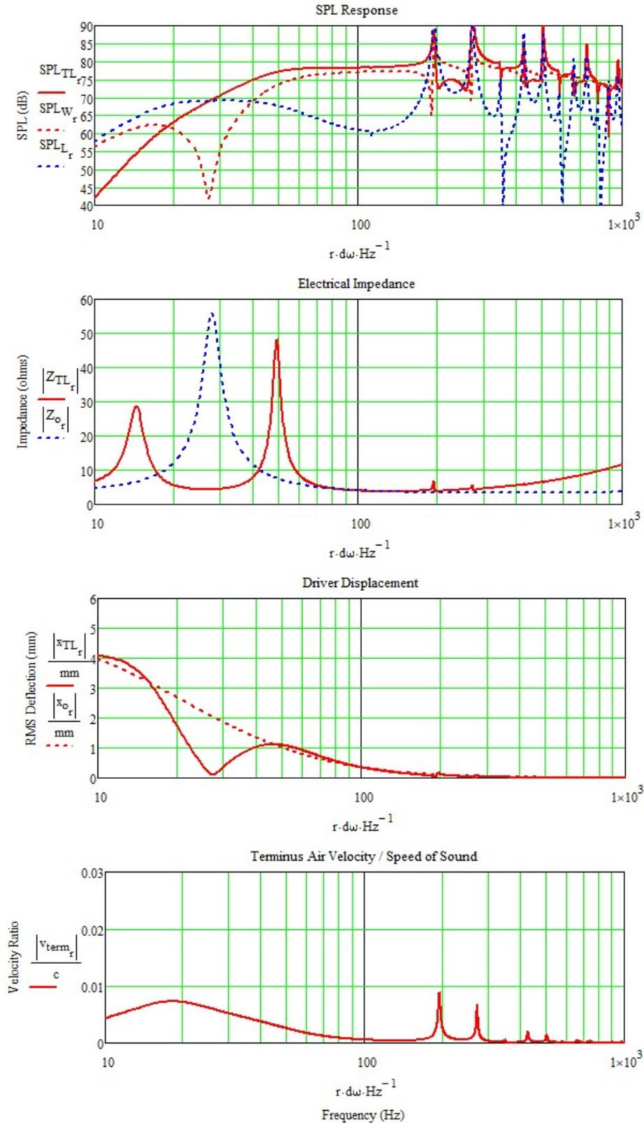
Figure 8 : Expanding 1:5 Transmission Line Enclosure w/o Fiber Stuffing
