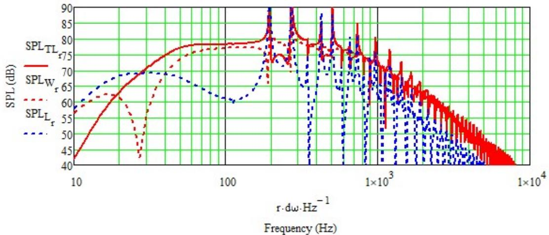
Figure 5 : Expanding Transmission Line Enclosure Results
