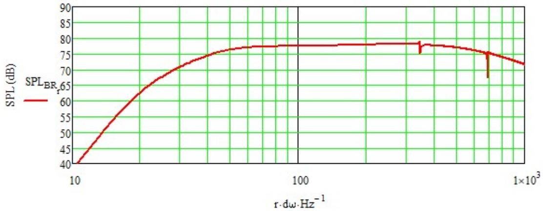
**SPL Response of a 10:1 Tapered Transmission Line Enclosure w/o Fiber Stuffing**
