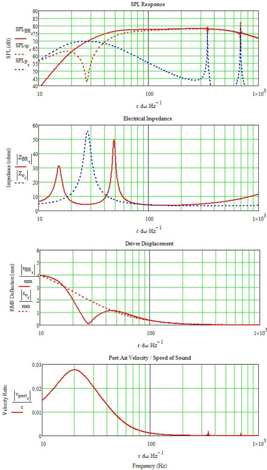
Figure 7 : Tapered 5:1 Transmission Line Enclosure w/o Fiber Stuffing
