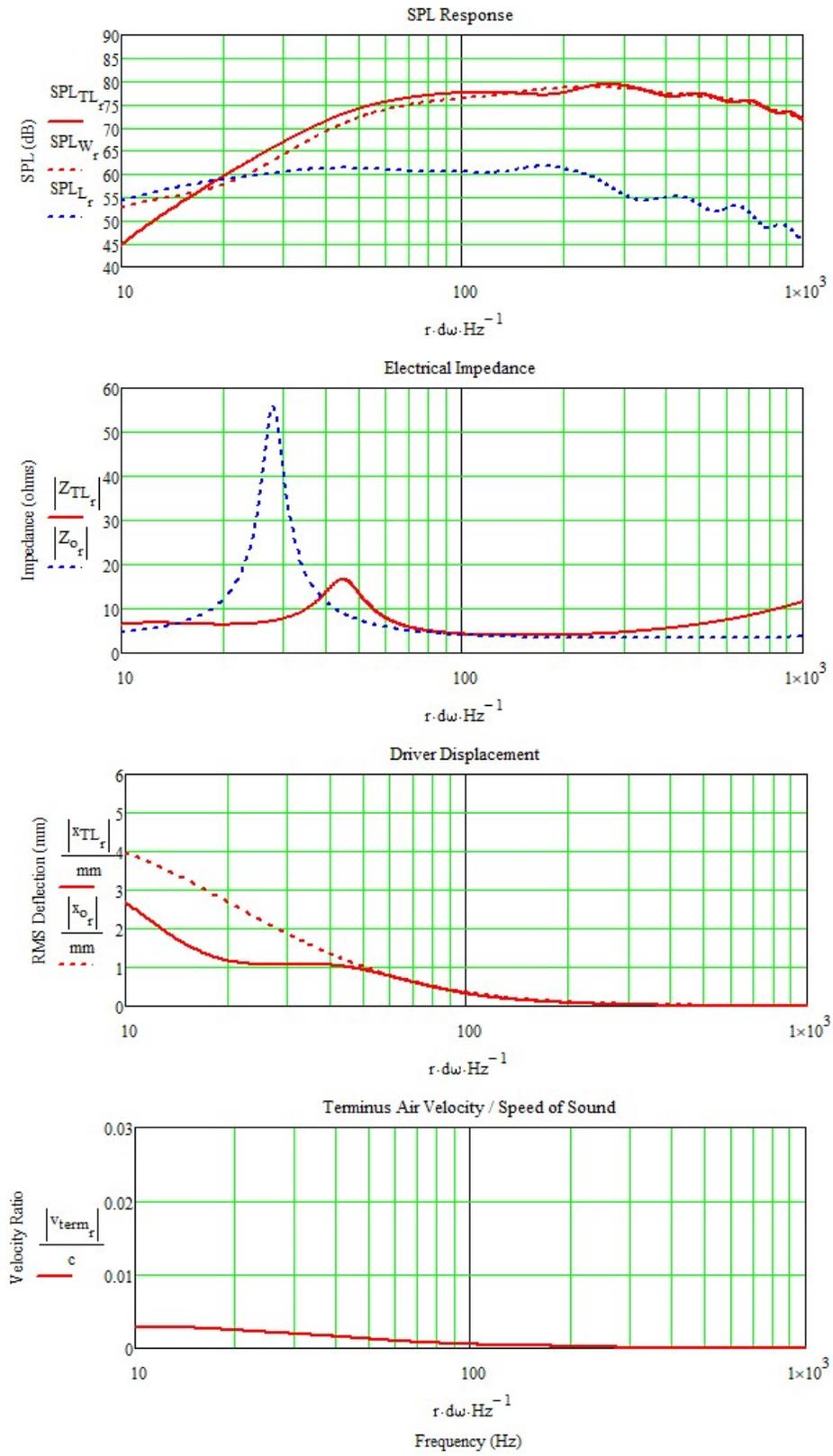
Figure 11 : Expanding 1:5 Transmission Line Enclosure w/ 0.5 lb/ft<sup>3</sup> of Fiber Stuffing
