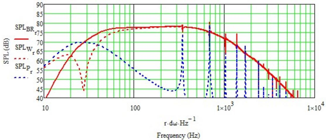
Figure 4 : Tapered Transmission Line Enclosure Results
