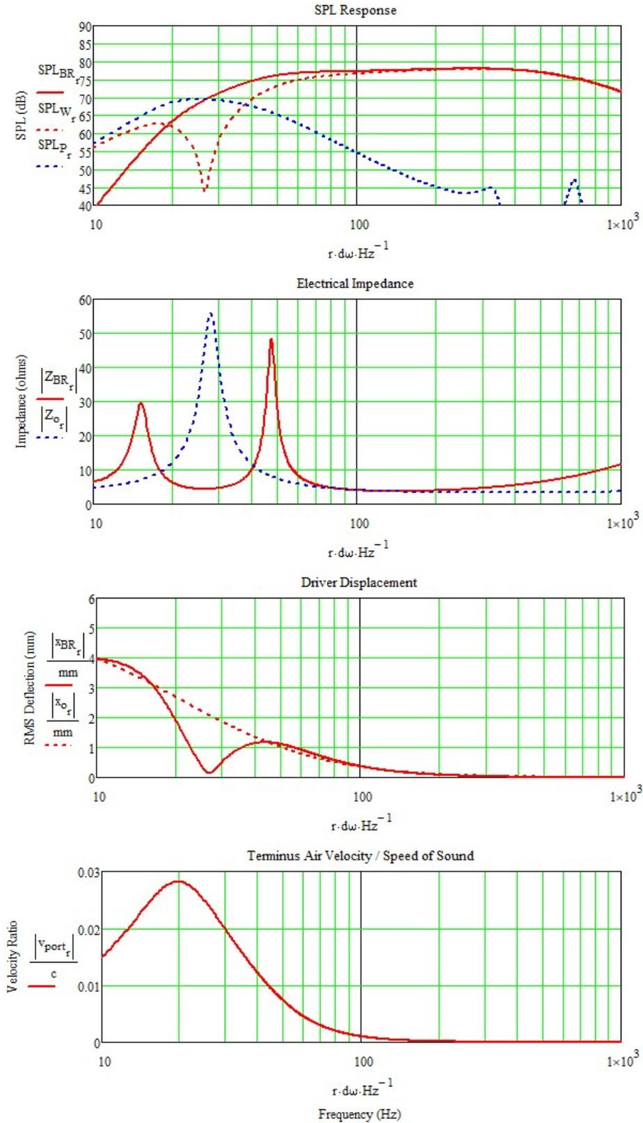
Figure 10 : Tapered 5:1 Transmission Line Enclosure w/ 0.5 lb/ft<sup>3</sup> of Fiber Stuffing
