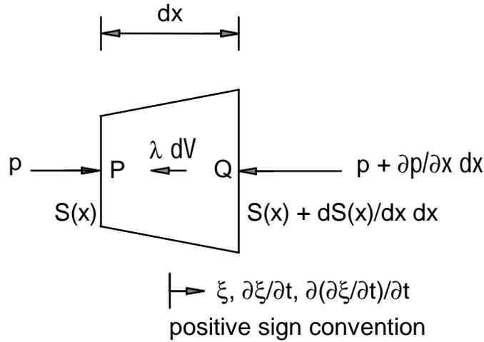
The figure depicts the pressures acting on each face, the damping coefficient  $\lambda$  acting on the volume, and the positive sign convention for the displacement, velocity, and acceleration. Summing the forces acting on the air mass and setting the result equal to the inertial acceleration results in the equation of motion.
