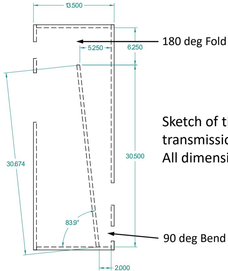
Sketch of the 5:1 tapered Satori transmission line speaker enclosure. All dimensions are in inches.
