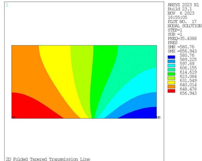
The plots above show the pressure profile in the Satori TL enclosure for the quarter wavelength standing wave at the tuning frequency of approximately 35 Hz. The left plot shows the entire enclosure while the right plot only shows the 180-degree fold at the top of the enclosure. These are normalized result. The pattern/distribution is important, but the absolute pressure magnitudes are meaningless.
