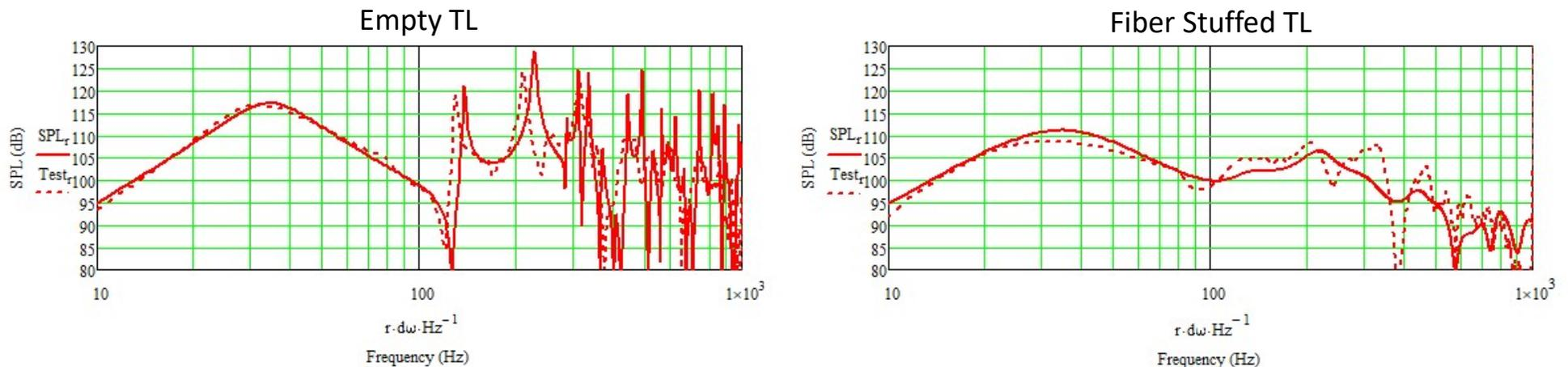
The two plots shown above contain the calculated (solid red curve) and measured (dashed red curve) terminus near field SPL responses. Correlation has improved with the advanced corner modeling (10 parallel paths used) method. There are more peaks and dips seen in the empty TL calculations and the roll off previously observed in the measurements above 300 Hz is now predicted.
