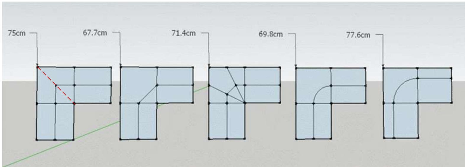
I lifted this picture from the Internet. I do not know its origin, but it is referenced on many on-line forums and discussion groups. When I model a TL, I use the left-hand method (the centerline method) with the addition of a diagonal (red dashed line) across the corner. Hornresp users tend to favor the middle modeling method (the advanced centerline method).
