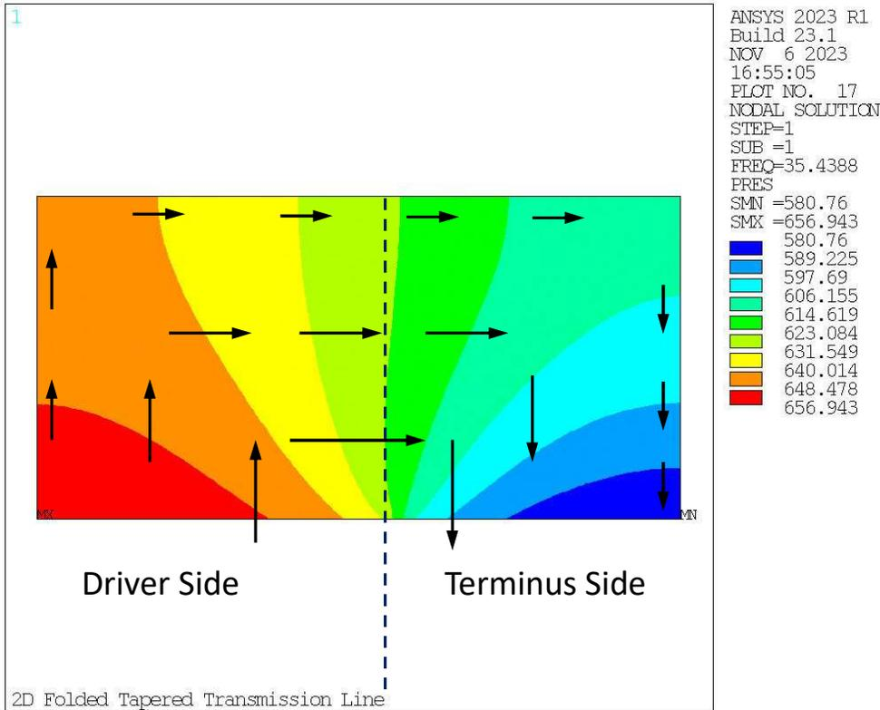
Looking at the pressure gradient as it transitions through the 180-degree fold you can see a fan-like pattern. The pressure gradient along the inside of the fold is much higher than the gradient along the outside of the fold. Estimating and sketching in oscillating velocity arrows shows the non uniform velocity profile when moving outward along a cross-sectional areas.
