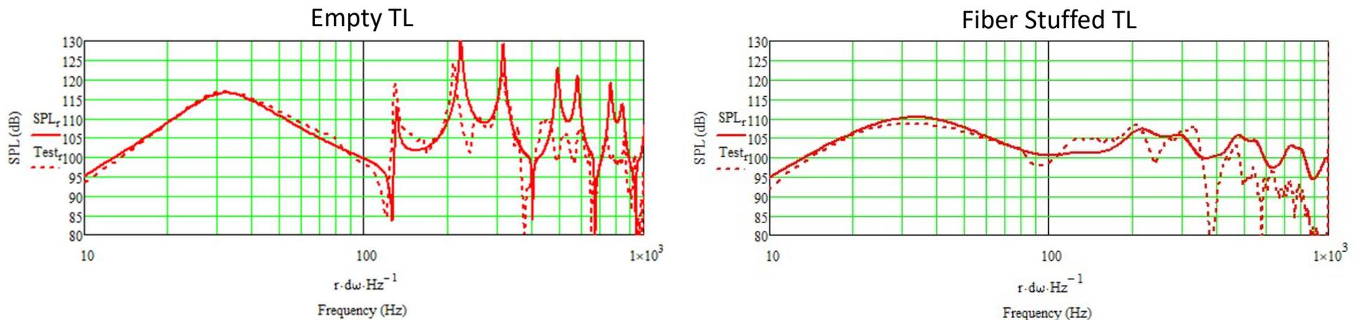
The two plots shown above contain the calculated (solid red curve) and measured (dashed red curve) terminus near field SPL responses. The calculated results use the centerline model to represent the 180-degree fold and 90-degree bend.
