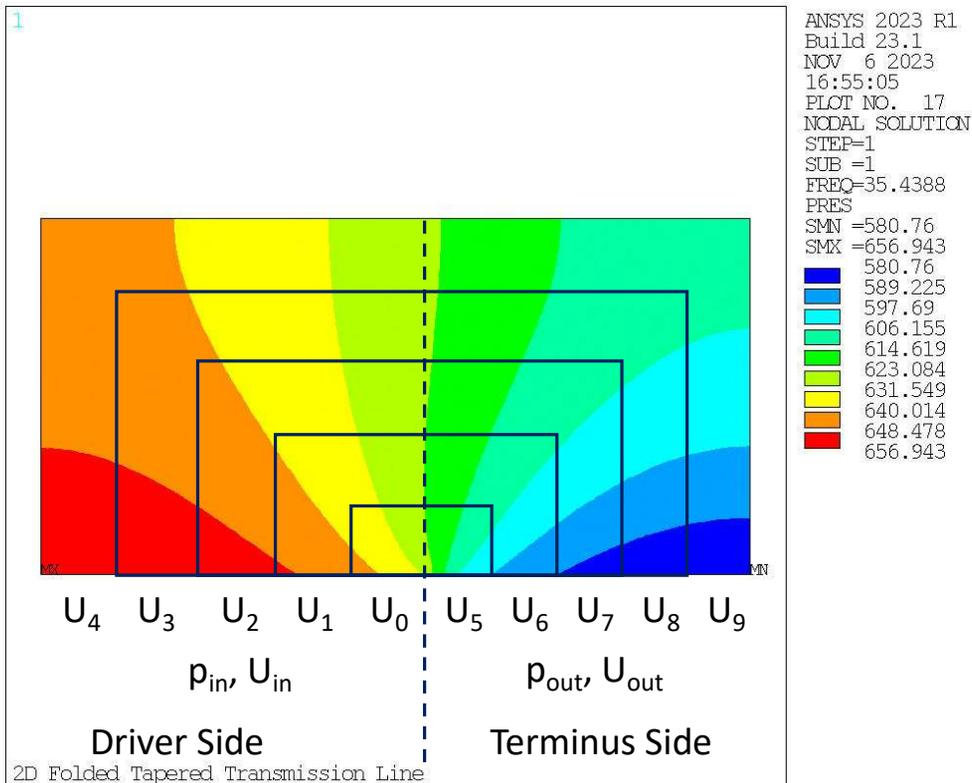
The advanced corner modeling method breaks up the fold into many parallel paths. The pressures,  $p_{in}$  and  $p_{out}$ , at each end of the different paths on each side of the fold are assumed to be uniform while the different volume velocities in the paths are the unknowns. The sum of the different path volume velocities on each side equal  $U_{in}$  and  $U_{out}$  respectively.
