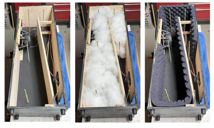
Examples of the Satori TL enclosure just before final assembly. Fiber or Foam were applied to the same portion of the TL's length, approximately the first 3/4 of the tapered enclosure.
