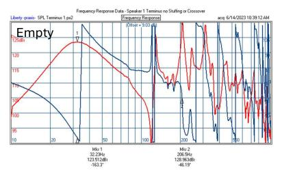
The terminus output determines the speaker's bass performance. Comparing the foam and fiber plots shows that a 0.5 lb/ft^3 density of fiber significantly reduced the peaks and dips compared to an acoustic foam lining. To replicate the peaks and dips of the acoustic foam required the stuffing density in the fiber model to be reduced by a factor of 10 to 0.05 lb/ft^3. A fiber density of 0.05 lb/ft^3 is extremely sparse.
