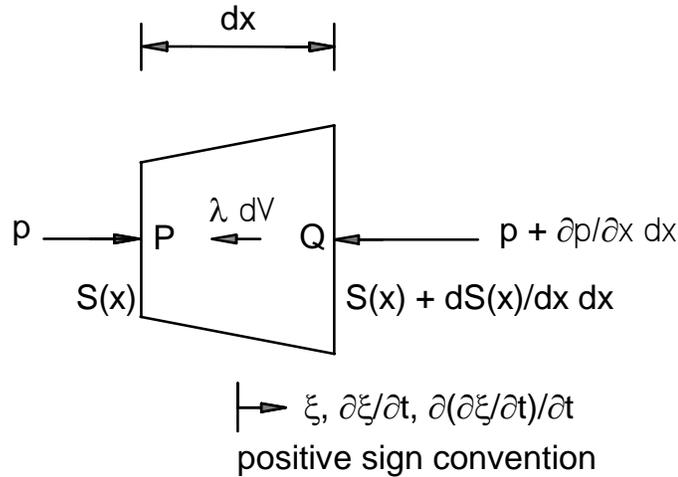
The figure above depicts the pressures acting on each face, the damping coefficient  $\lambda$  acting on the volume, and the positive sign convention for the displacement, velocity, and acceleration. Summing the forces, and setting the result equal to the inertial acceleration, results in the equation of motion.
