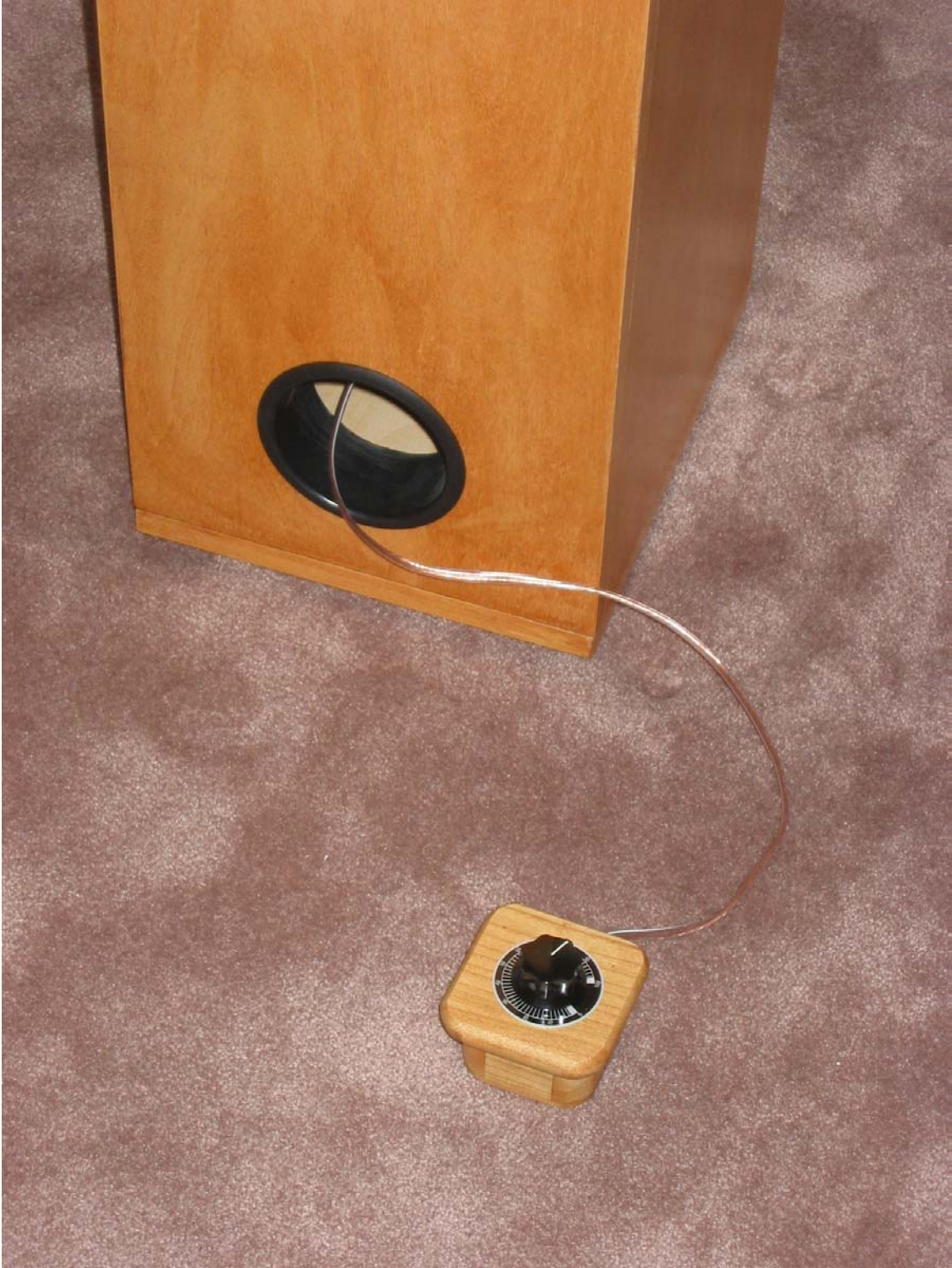
Figure 4 : Installed Variable Resistor
