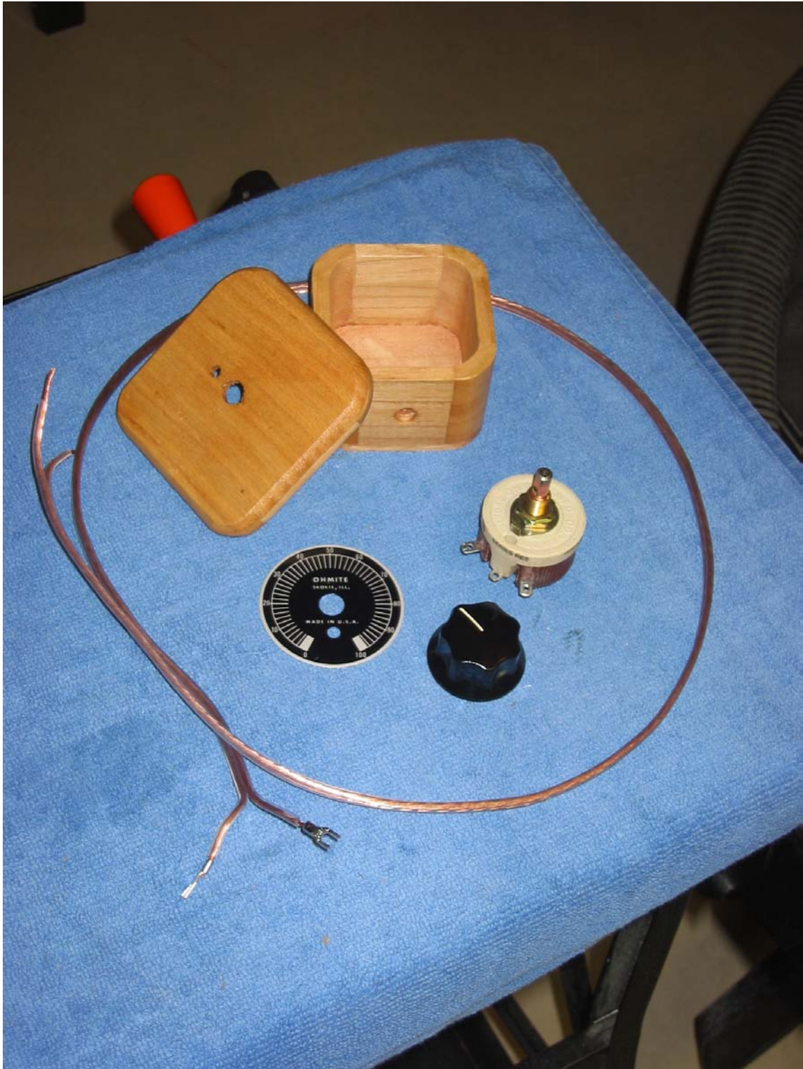
Figure 2 : Variable Resistor Parts
